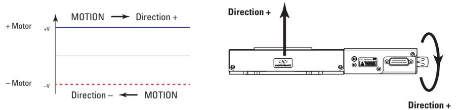
In the above drawings, + Motor signal is referred to - Motor signal.
