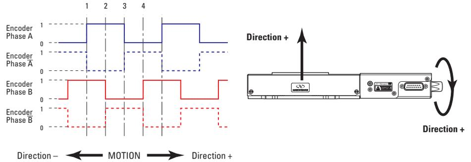
The incremental sensor consists of an optical scale and an encoder head. When the carriage moves, the encoder head generates square signals in quadrature and sends to pins #6, #7, #13 and #14 of the SUB-D15 connector.
